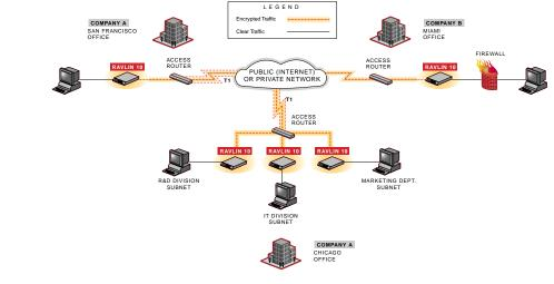
Using Ravlin to establish Secure Intranets, Secure Extranets and Secure Remote Access.
